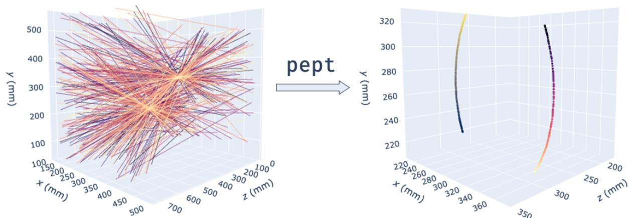
Transforming gamma rays, or lines of response (left) into individual tracer trajectories (right) using the *pept* library. Depicted is experimental data of two tracers rotating at 42 RPM, imaged using the University of Birmingham Positron Imaging Centre’s parallel screens PEPT camera.
