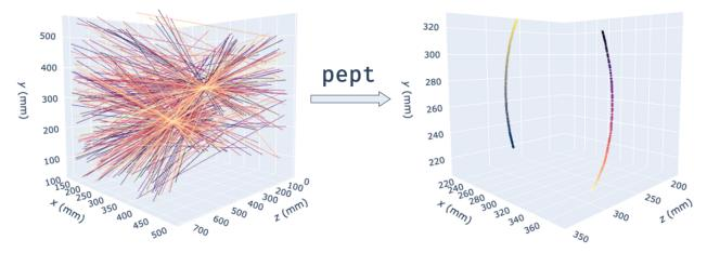
Transforming gamma rays, or lines of response (left) into individual tracer trajectories (right) using the *pept* library. Depicted is experimental data of two tracers rotating at 42 RPM, imaged using the University of Birmingham Positron Imaging Centre's parallel screens PEPT camera.
